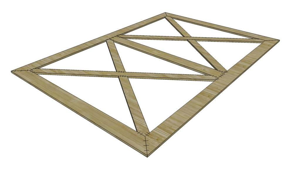
As a next step, take 1x10 T&G boards and fasten with screws, keeping all edges flush with outside trims. Make sure to fasten screws into all trims & cross-bucks. This gives your door clean look, without any screws visible from outside.
