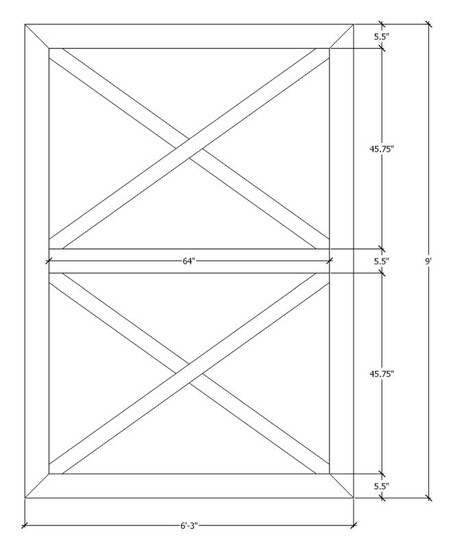
12'-6"x9' Split Slider Assembly Assembly of Outside Trim - Step #1
