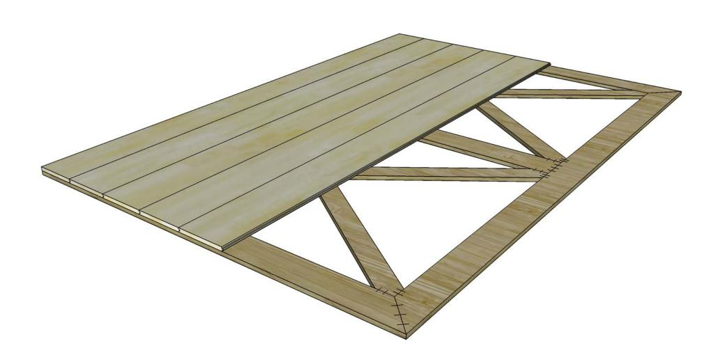
Next, fasten 5.5" wide inside trim flush with outside edges and one in center of door. As an option, you may also fill this door with wood in between trims.
